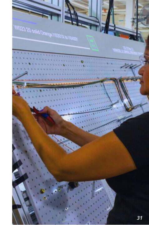
[LightGuide] puts work instructions exactly where you build your product, so you're reducing time looking at printed instructions by putting the focus exactly where operators' attention should be.
